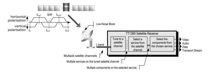
Figure 1.4: What the Satellite Receiver Does
